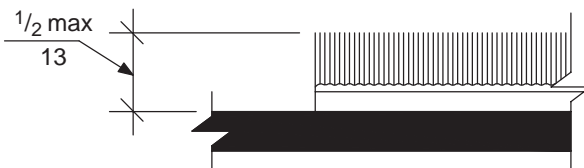
Fig. 302.2 Carpet on Floor or Ground Surfaces
