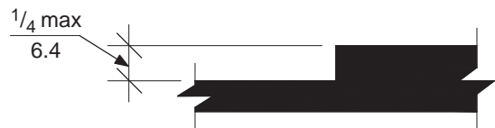
Fig. 303.2 Vertical Changes in Level
